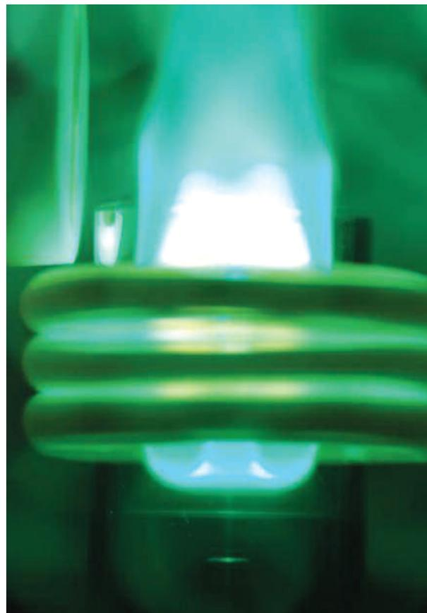
Figure 1: Plasma aspirating naphtha after auxiliary and nebulizer gas flows have been optimized.
